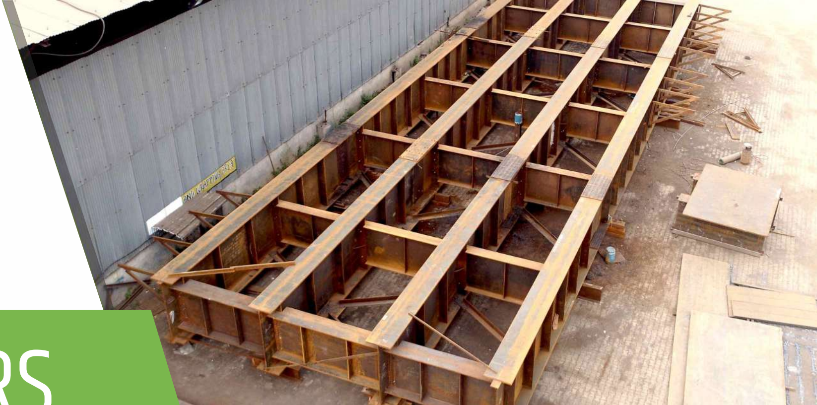
Project : PWD Orissa Girder Type : ROB Composite Girders Span : 25.49 M X 12
